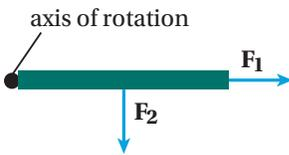
34. Two forces equal in magnitude but opposite in direction act at the same point on an object. Is it possible for there to be a net torque on the object? Explain.
