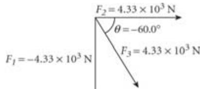
**2. PLAN** Select a coordinate system, and apply it to the free-body diagram: Let  $F_1$  lie along the negative  $y$ -axis and  $F_2$  lie along the positive  $x$ -axis. Now  $F_3$  must be resolved into  $x$  and  $y$  components.
